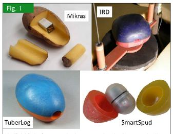
Artificial fruits for measuring impact acceleration in processing lines of agricultural products (Fotos: ATB)
