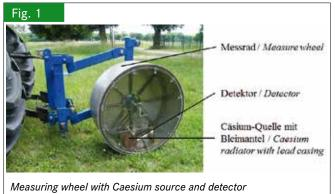
Measuring wheel with Caesium source and detector (Foto: Geyer, ATB)
