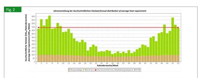
Annual distribution of average heat requirement of 500  $kW_{el}$  biogas plant incl. 80 single-family houses (built 1978 to 1995) and idealised heat supply from a biogas plant (red line)
