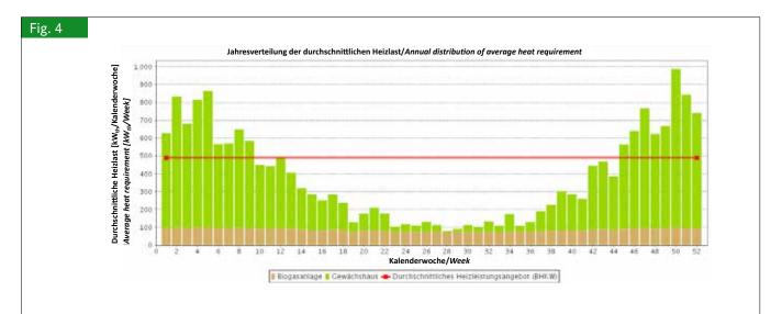
Annual distribution of average heat required from a 500 kW<sub>el</sub> biogas plant incl. 10,000 m<sup>2</sup> greenhouse and idealised heat production of biogas plant (red line)
