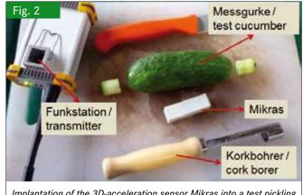
Implantation of the 3D-acceleration sensor Mikras into a test pickling cucumber (Foto: J. Surdilovic)
