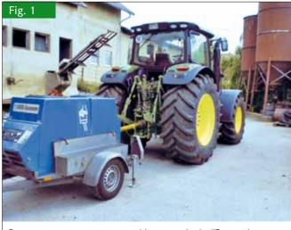
Dynamometer measurement - eddy current brake "Eggers dynamometer" at the PTO (Foto: Reckleben)
