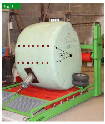
Silage Bale at the density test bench and position of the measuring points (Foto: Maack)
