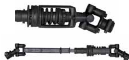
Original IHC PTO drive shaft with axial ratchet clutch, ca. 1950
