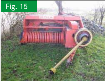
Coil-spring friction clutch 550 Nm, year of construction 1958
