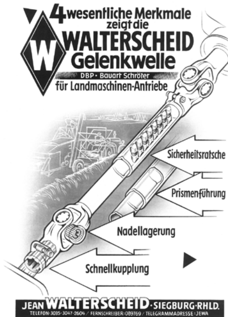
PTO drive shaft with integrated overload clutch, brochure 1953
