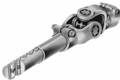
Cam-type ratchet 400 Nm, year of construction 1953/54
