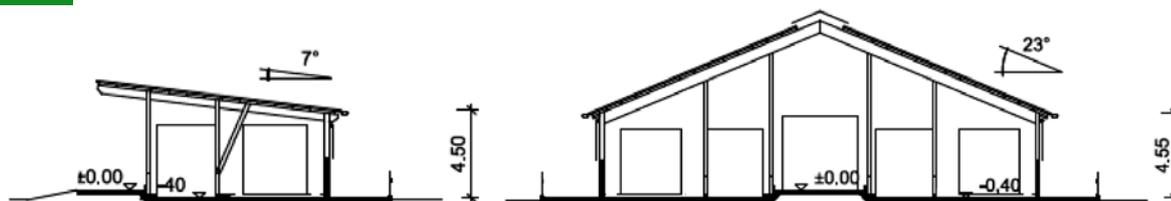
Litter system, sectional drawings: one row assembly with single pitch roof (left) and two row assembly with double pitch roof (right)
