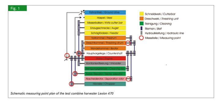
For the recording of the torque, strain gages were used. Hall-sensors deliver the rotation speed. The signals of the sensors are digitized by the rotor electronic and transmitted through an aerial without any contact. In the receiver, both torque and the rotation speed are converted in to CAN-messages and passed on the measuring-CAN-bus.
