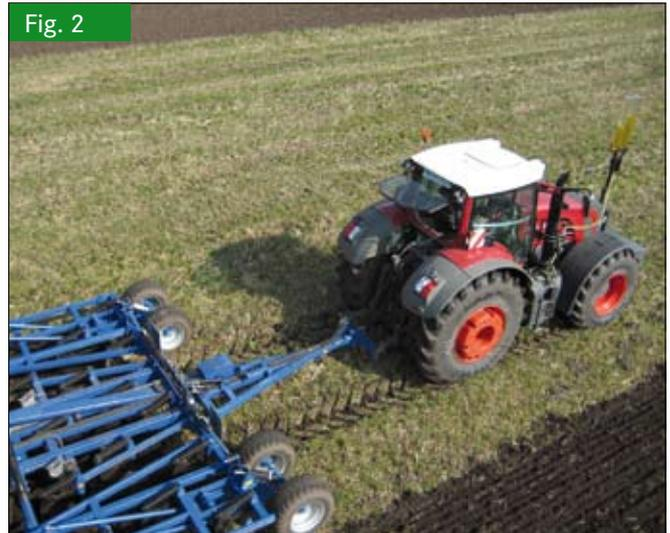
Fig. 2: Adjusted tire inflation pressure (pictured: 0.6 bars) results in less soil deformation and more driver comfort
