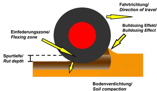
Fig. 1: Rolling on soft ground is an energy consuming process: tire deformation and bulldozing cost an extra 10% of diesel fuel with every additional centimeter of rut depth
