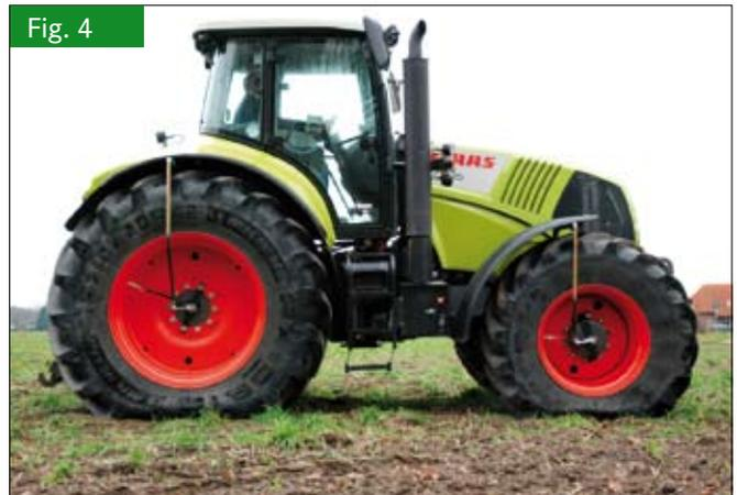
Fig. 4: Backfitted „Strotmann“ Central Tire Inflation System (CTIS) (appr. 2.500 €) with air hoses above the fenders. System functions are centrally managed with the StG-Terminal
