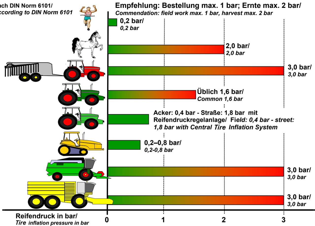
Fig. 3: 1 bar for seeding and 2 bar tire inflation pressure for harvesting should be the maximum tire pressure
