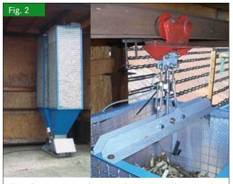
Fig. 2: Sample container for drying of wood chips (left), registration of weight loss by a load cell (right)
