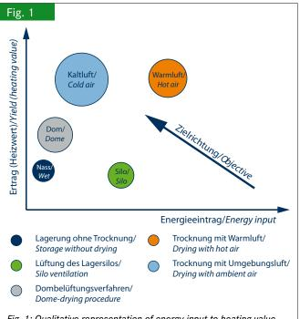
*Fig. 1: Qualitative representation of energy input to heating value during the drying process of wood chips*
