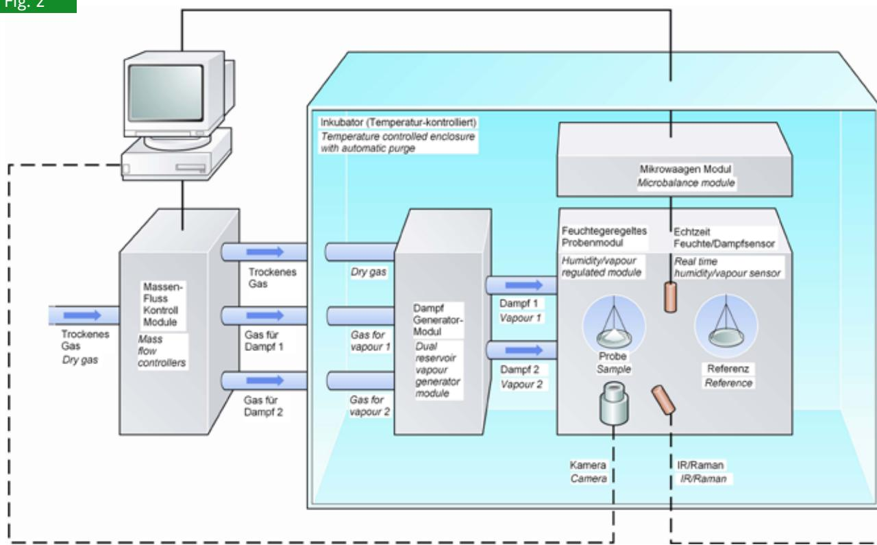
Fig. 2: Schematic diagram and principle of the dynamic water vapour sorption apparatus
