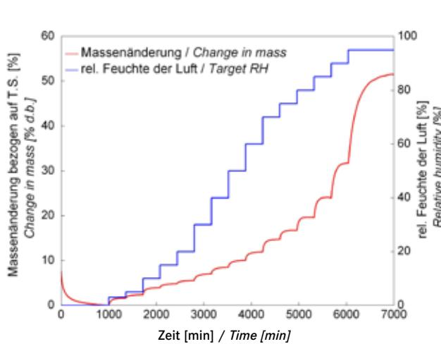
Fig. 3: Drying curve and equilibrium moisture adsorption profile of *M. officinalis* exposed to different values of relative humidity at 25 °C
