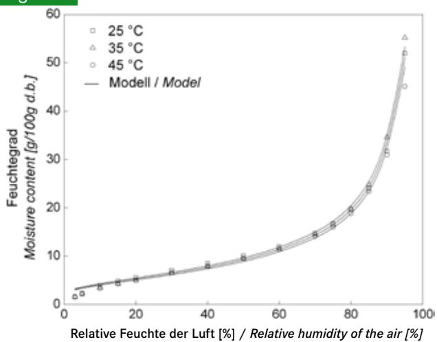
Fig. 5: Adsorption isotherms of *M. officinalis* fitted by Halsey-model
