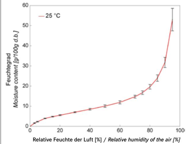
Fig. 4: Adsorption isotherm of *M. officinalis* at 25 °C
