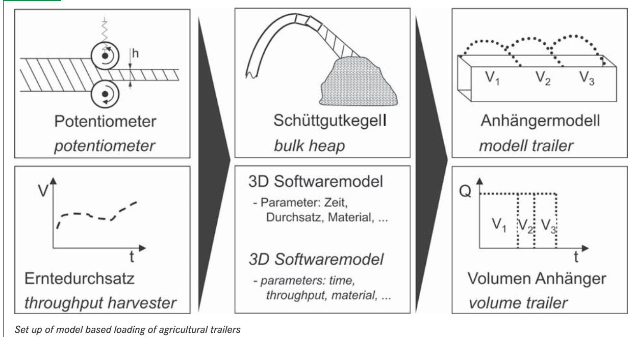
divided into several discrete volume spaces. By generating and achieving loading points the discrete spaces are to be filled up to the maximum load of the trailer. Regarding the throughput and the effective loading position a software model estimates the loading state inside the trailer, until it is filled at maximum rate. **Figure 1** depicts the set up principle.
