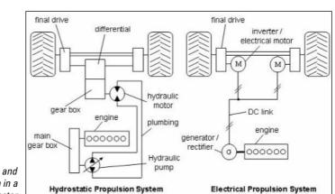
Fig. 3: Hydrostatic and electrical propulsion in a combine harvester
