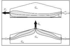
Fig 3: Fresh air is sucked in from outdoor through the stable, whereas the contact to the inner stable emissions areas is very different. It is intensive with cross flow (at the top) and low by extraction over the ridge.
