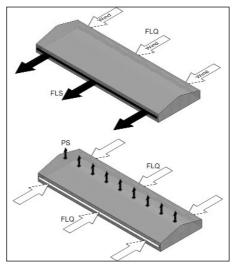
Fig 2: The sides of outgoing air are marked by black colour: Area sinks (FLS) and point sinks (PS). The upper case characterizes a cross flow by free ventilation, the case below a forced ventilation over the ridge. The air goes in by area sources (FLQ).
