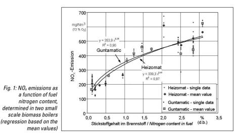
Due to unstable wood pellet prices and a beginning discussion about the availability of raw materials for pelleting, it seems appropriate to use agriculturally produced biomass also in residential boilers. For such non-wood fuels (straw pellets, grain kernels, energy plants), new boilers are currently being developed or are already being offered. In a research project, such kinds of utilization were investigated by means of practical combustion tests.
