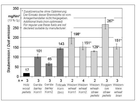
Fig. 3: Total dust emissions using various biofuels (without lime added) in a 30 kW furnace (Guntamatic Powercorn 30) at maximum heat load (n = number of measurements)
