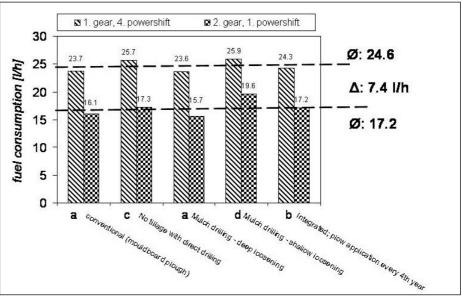
Fig. 3: Fuel consumption at subsoiling in different soil-tillage systems for two driving strategies. Miniscules indicate significant difference (Student-Newmann-Keuls-test;  $\alpha$ =0.05) in fuel consumption in dependence of the soil-tillage system
