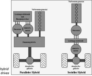
Fig. 1: Schematic diagram of hybrid
