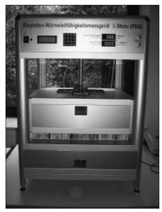
Fig. 2: Measuring the thermal conductivity
