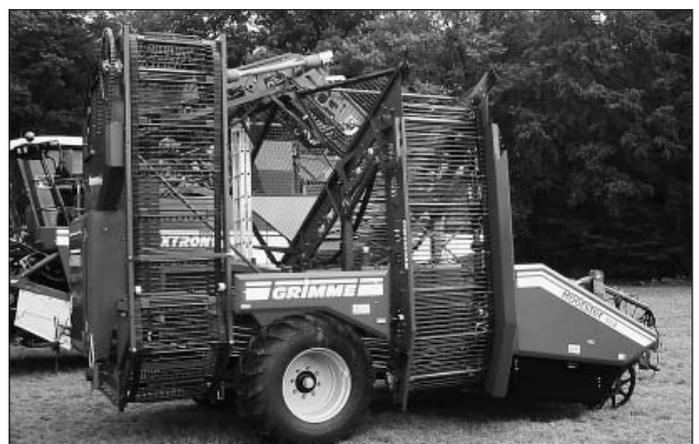
*Fig. 3 and 4: Reduced to the minimum: Grimme developed especially for Eastern European demands the pulled high-capacity beet-top mulcher BM330 (left) and the six-row pulled beet harvester Rootster 604 with a 4-t loading hopper*
