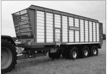
Fig. 2: Bergmann has adjusted its trailer HTW 65 for chopped forage to the increased capacities of the forage harvesters: 65 m3 loading volume and a hydraulic Tridem travelling gear are the insignia.
