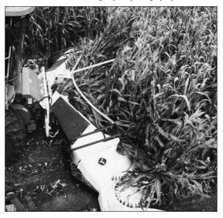
Fig. 3: Kemper has developed the row-independent cutting head Champion 475 for the harvest of high-yielding energy maize
