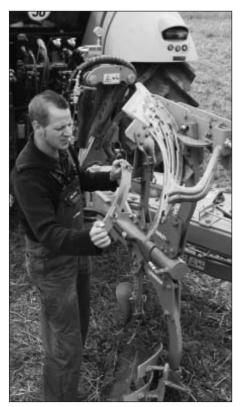
Fig. 2: In the DuraMaxx system from Lemken, wearing parts can be replaced without tools
