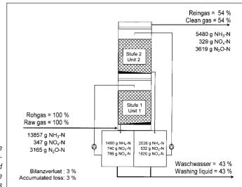
Fig. 3: Nitrogen balance of a two-stage, wateroperated scrubber used for the cleaning of waste air from piggeries
