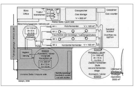
Fig.1: Scheme of the pilot-biogas plant with four horizontal cylindrical fermenters (each 165 m<sup>3</sup>), one second stage fermenter (vertical cylinder with 1000 m<sup>3</sup>) and gasmotor (511 kW<sub>eb</sub> 615 kW<sub>th</sub>) cogeneration unit
