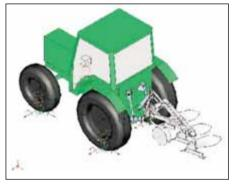
Fig. 8: Construction of simulation models (Mechanica – model for tractor implement system; tractor: John Deere 6400; implement: plough
