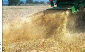
Fig. 1: Visible differences of straw distribution of test chopper with modification on one side
