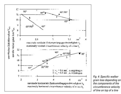
the associated reduction in time spend by the material in the separation system and reduced impulse transmission, led to substantially higher grain losses. *Figure 4* confirms these relationships using the example of the tine chain walker.
