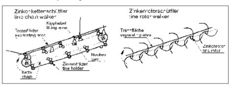
Fig. 1: Working principles tine chain walker – tine rotor walker
