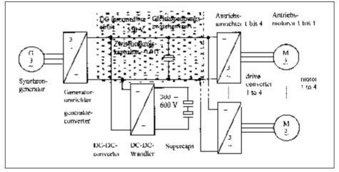
Fig. 1: Coupling the ultracap's on the intermediate circuit
