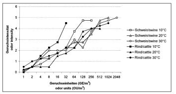
Fig. 2: Intensity of odor perception above the odour threshold of swineand cattle-slurry at different temperatures
