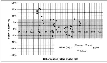
Fig. 2: Relative error of the bale mass with different bale masses
