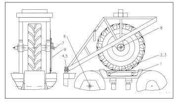
Fig. 1: Flat-belt tyre test stand
