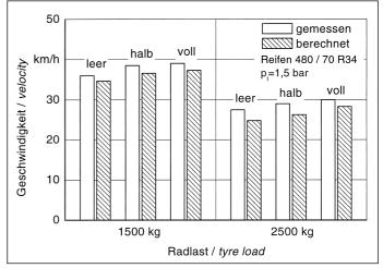
Fig. 3: Variation of the critical velocity for different filling levels
