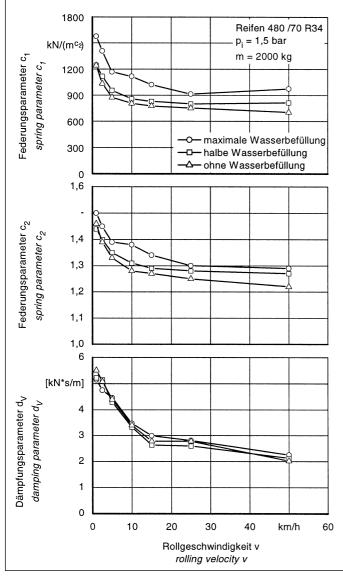
Fig. 2: Impact of the water ballast on the tyre parameters
