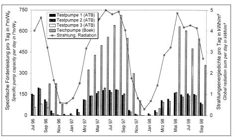
Fig. 1: Yearly courses of the specific pump capacity of different pv-pumps in a monthly average
