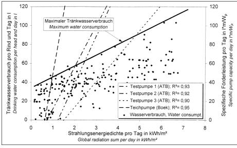
Fig. 2: Drinking water consumption of non-lactating cows and specific capacity of pv-pumps versus global solar radiation intensity
