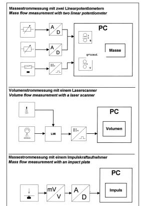
Fig. 2: Measuring systems of determining throughput
