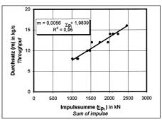
Fig. 5: Measuring mass flow with an impact plate
