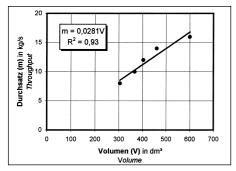
*Fig. 4: Measuring volume flow with a laser-scanner*
