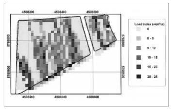
Fig.2: Local distribution pattern of soil load caused by grain transport
