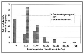
Fig.3: Histogram of the load index for two field vehicles
