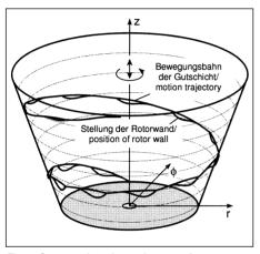
Fig. 2: Computed motion trajectory of rotary cleaning system
