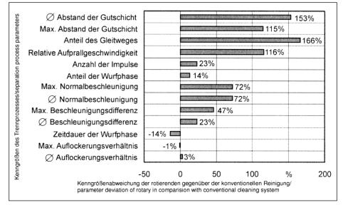
Fig. 4: Parameter deviation of rotary in comparison with conventional cleaning system
