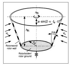
Fig.1: Stucture of rotary cleaning system
