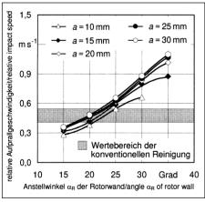
Fig. 3: Relative impact speed of rotary cleaning system
